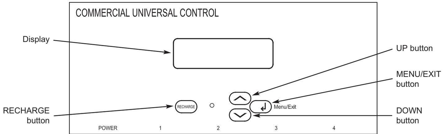
The CUC2 is a menu-driven electronic controller with a dot matrix display. The UP (▲) and DOWN (▼) buttons move the cursor (>) up and down the menu choices. The MENU/EXIT (←) button enters the value selected and returns the display back a level. The controller will return to the normal operating screen after 4 minutes, if left in a menu and no selection has been made.
