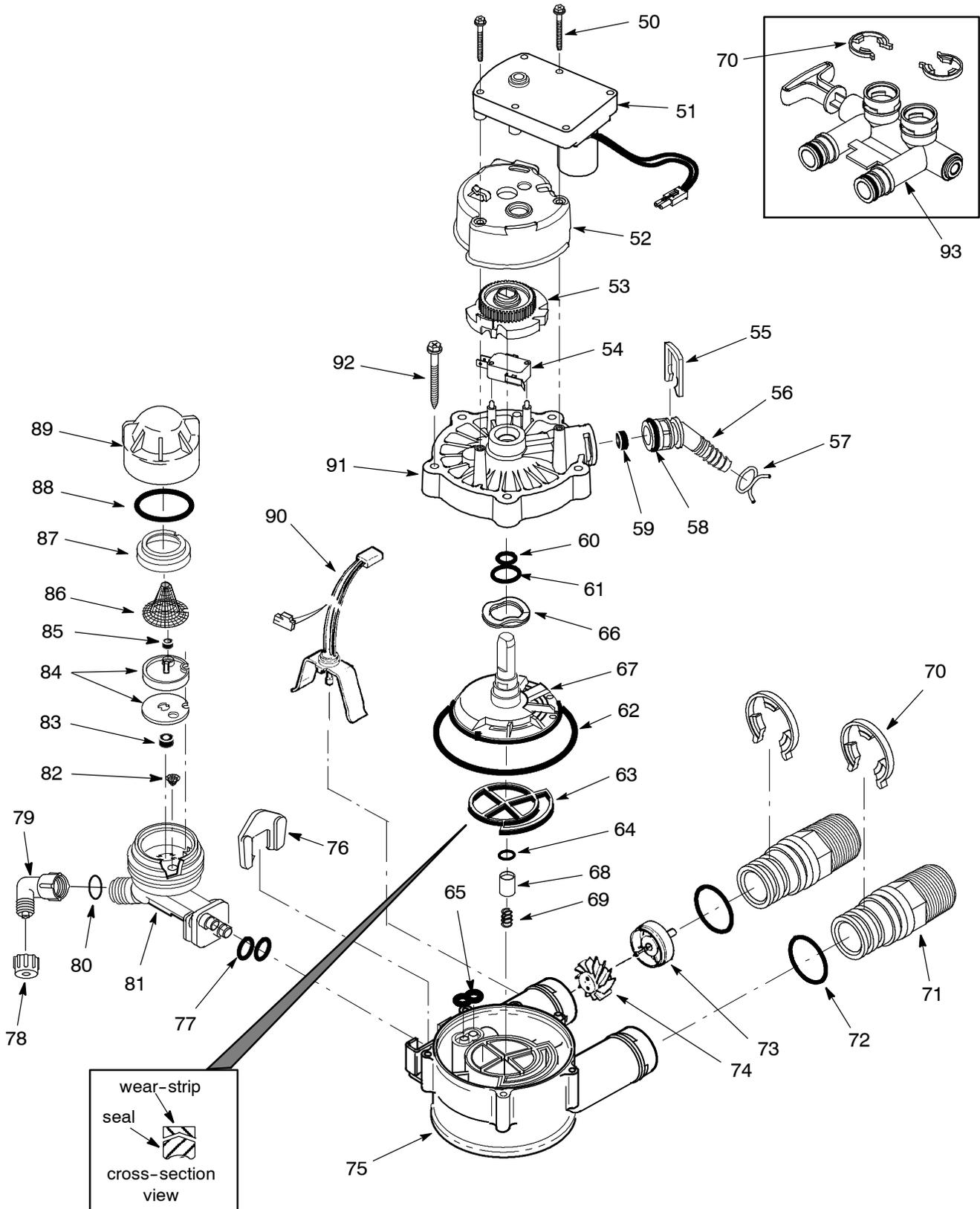
**VALVE REPAIR PARTS**
