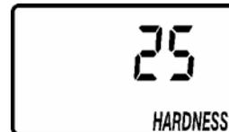
You can get the grains per gallon (gpg) hardness of your water supply from a water analysis laboratory, or call and ask your local water department, if you are on a municipal supply. If water contains iron, add to the water hardness at a ratio of 5 grains for each 1 ppm of iron.
