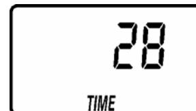
...Press the DOWN button to display the number of regenerations initiated by this face plate since the model code number was entered.
