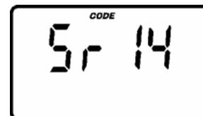
**For correct softener operation, the model code must be Sr14.**
