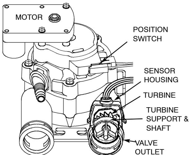
If you don't get a reading in the display, with faucet open, pull the sensor from the valve outlet port. Pass a small magnet back and forth in front of the sensor. You should get a reading in the display. If you get a reading, unhook the in and out plumbing and check the turbine for binding.
